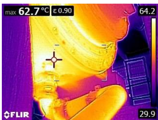
THERMOGRAPHY IMAGING OF GEARBOX
